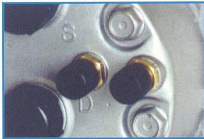
Figure 1. Charge and discharge chargers (C/C)
